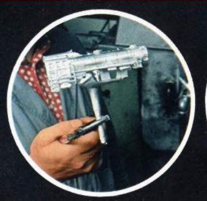
The castings are made by pressing molten zinc at 420° into the mold.
