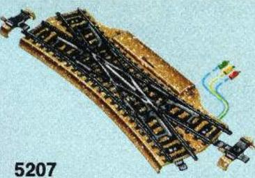
Double slip switch · Enables track spacing of 77.4 mm (3-1/16") to be maintained · Operated by double solenoid · Hand operating lever on actuator case Length of straight section 180 mm (7-1/8") . The curve is the same as for 5202, 5221 and 5206 · 2 make-up lengths 5208, each 8 mm (5/16") long, are included
