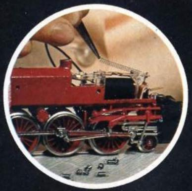
Precision operation: using tweezers to fit the reverser unit spring into the model.
