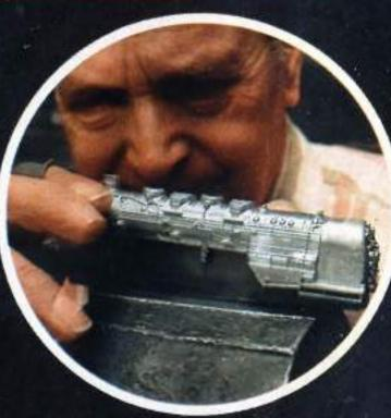
On each locomotive the casting burrs are smoothed off carefully by hand.
