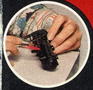
Only the basic color is applied by spraying machine; all details are hand-painted.
