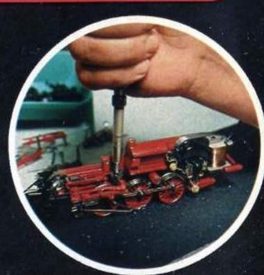
The driving rod assembly is screwed onto the frame with great care.
