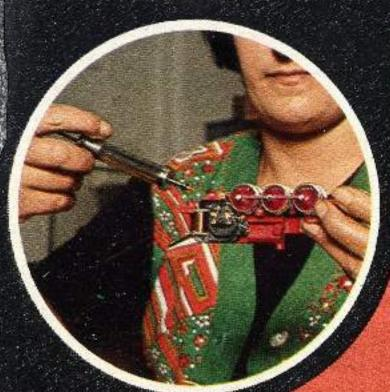
A drop of oil ensures that the gear wheels in the driving truck run smoothly.
