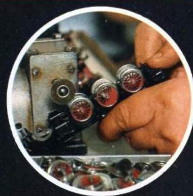
On fitting driving trucks it is important to carry out true-running tests.
